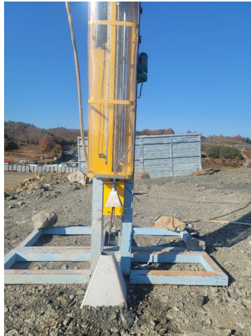
Fig. 2 Photograph of the AWJ drilling unit
